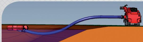
**ATTENTION:** Never use a grappling device to pull strainer from the water, this may cause damage of the floating chamber (2). Only use handles for this purpose!
